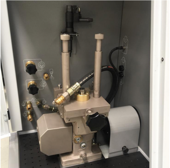
Patented Cam Box; stroke set between 10 & 18 mm.
